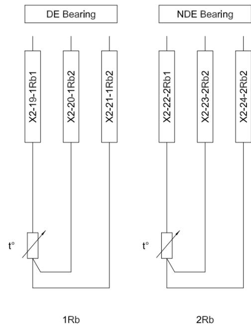
PT100 3 WIRES - 1 D.E. 1 N.D.E. BEARING
