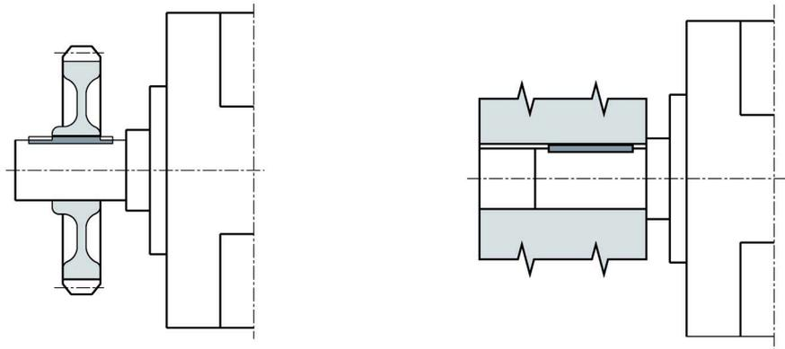
Align the offset at the coupling between electrical machines and the driven machines so that the maximum permissible vibration values according to ISO 10816-3 are not exceeded.
