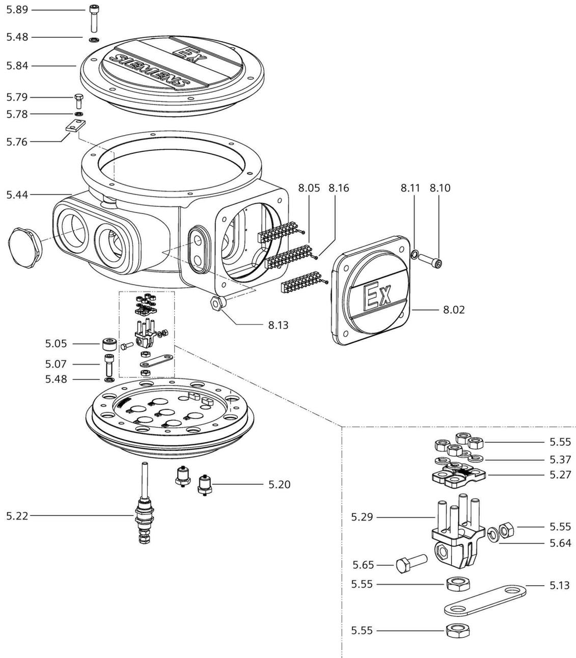
10.9.9 Auxiliary terminal box Ex eb optional, shaft heights 160 ... 355
