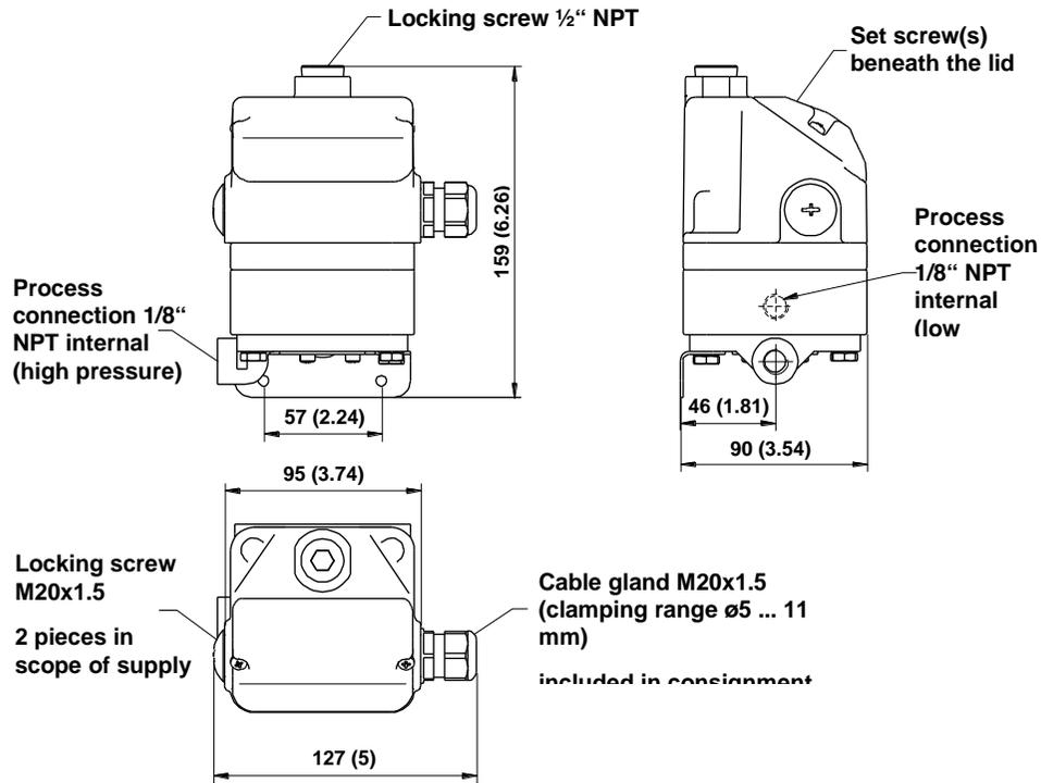
Fig. 8 Metal-diaphragm differential pressure switch type DPD1T .../DPD2T ...
