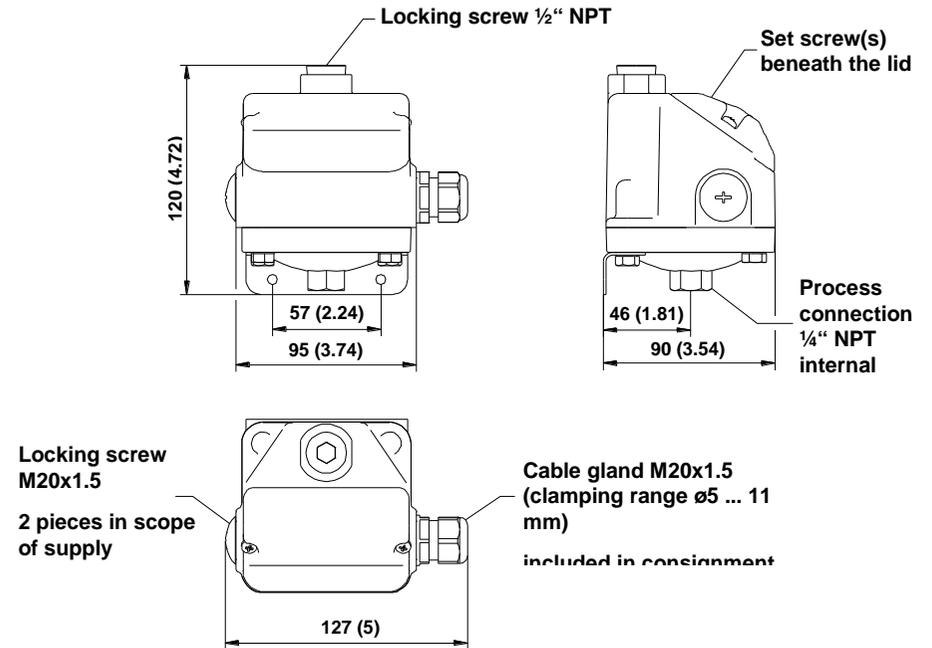
Fig. 7: Metal-diaphragm pressure switch type D1T .../D2T ...
