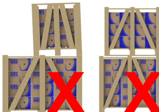
Figure 28 - Incorrect stacking
